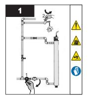
Close main water supply to the UV system, and then open a tap downstream of the UV System to release pressure.
